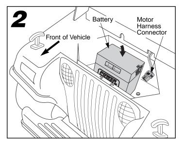
Place the Power Wheels® battery upright in the battery compartment.
